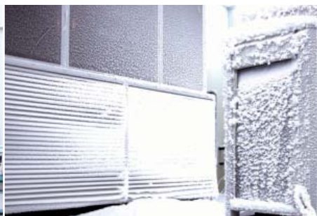
Environment simulation lab from -40°C - 55°C & snowfall simulation
