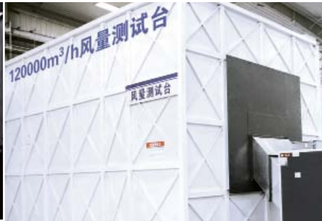
The largest air volume test platform in the industry (120,000 m³/h)
